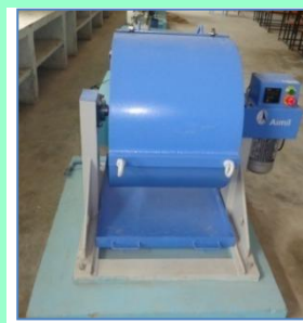
Los Angeles Abrasion testing machine
