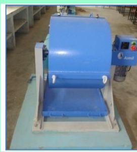
Los Angeles Abrasion testing machine
