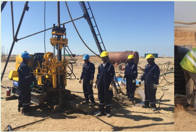
Figure 4: Soil investigation using borehole drill rigs
